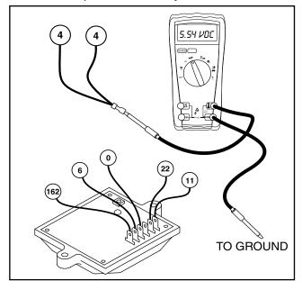
Figure 3. Field Boost Test Points
